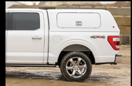
100SCC with optional flush side painted access doors for easy reach and a streamlined appearance.
